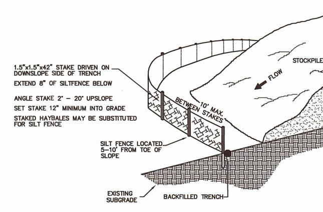
SILT FENCE @ TOE OF SLOPE APPLICATION
