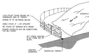
SILT FENCE @ TOE OF SLOPE APPLICATION
