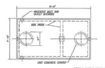
PROVIDE POSITIVE GRADE AWAY FROM MANHOLE COVER TO PREVENT GROWNWATER FROM ENTERING CHAMBER <u>PLAN</u> FINISHED GRADE ENGHED GRADE - 3° VENT -A 3" VENT -CUILET LIQUID LEVEL — CONTINUOUS HOT 4" DUTLET BAFFLE WITH FILTER " A" SCHEDULE #40 INLET BAFFLE DEFLECTOR-5'-a\* CROSS SECTION
