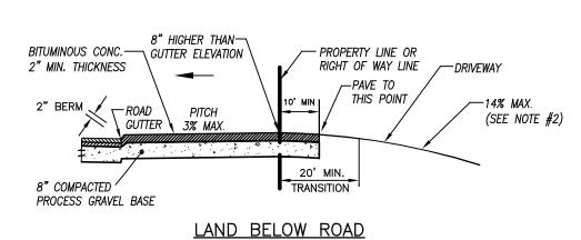
1. THE ABOVE DETAIL IS ILLUSTRATIVE ONLY AND DOES NOT APPLY TO EVERY SITUATION. REVIEW YOUR DRIVEWAY PERMIT FOR YOUR SPECIFIC REQUIREMENTS. 2. DRIVEWAYS IN EXCESS OF 10% GRADE, AND ALL COMMON (SHARED) DRIVEWAYS SHALL BE PAVED WITH BITUMINOUS CONCRETE.
