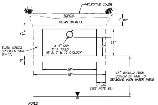
VENTING REQUIRED WHEN MORE THAN 18" OF COVER AS MEASURED FROM THE TOP OF THE UNIT TO FINISHED 2. FOR SYSTEMS INSTALLED IN FILL, CONTRACTOR SHALL PROVIDE 5' OF SELECT FILL OR ASTM C-33 SAND 5' AROUND PERIMETER OF SYSTEM.
