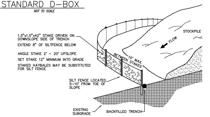
SILT FENCE @ TOE OF SLOPE APPLICATION
